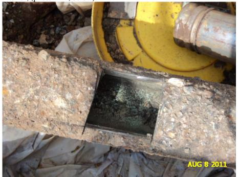
A11: Close-up of former 4-inch diameter Chromate wastewater conveyance pipe – cut open for inspection/cleaning.
