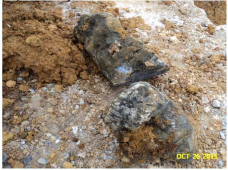
A35: View of two pieces of weathered limestone rock removed from the bottom of the vapor degreaser excavation at approximately 23' bgs.
